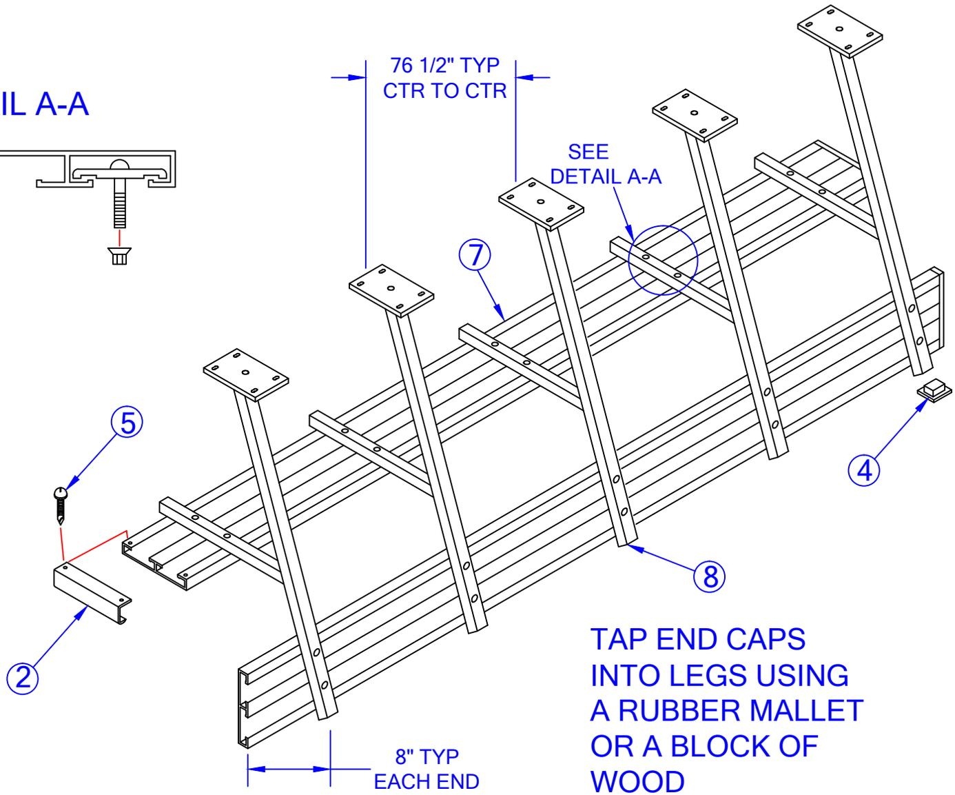
TAP END CAPS INTO LEGS USING A RUBBER Mallet OR A BLOCK OF WOOD
